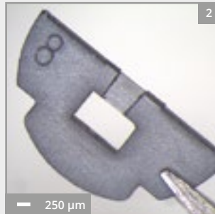
Fig. 1: Advanced Chunk (total length: 3.2 mm) with multiple lamellas from an IC-device (size of lamellas: 150 μm x 50 μm x 10 μm)
