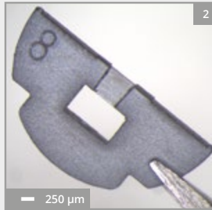
Fig. 1: XL-chunk (total length: 3.2 mm) with multiple lamellas from an IC-device (size of lamellas: 150 μm x 50 μm x 10 μm)
